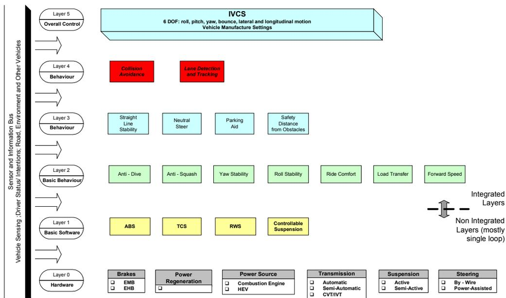
Fig. 8. Multi-layered vehicle control design architecture
