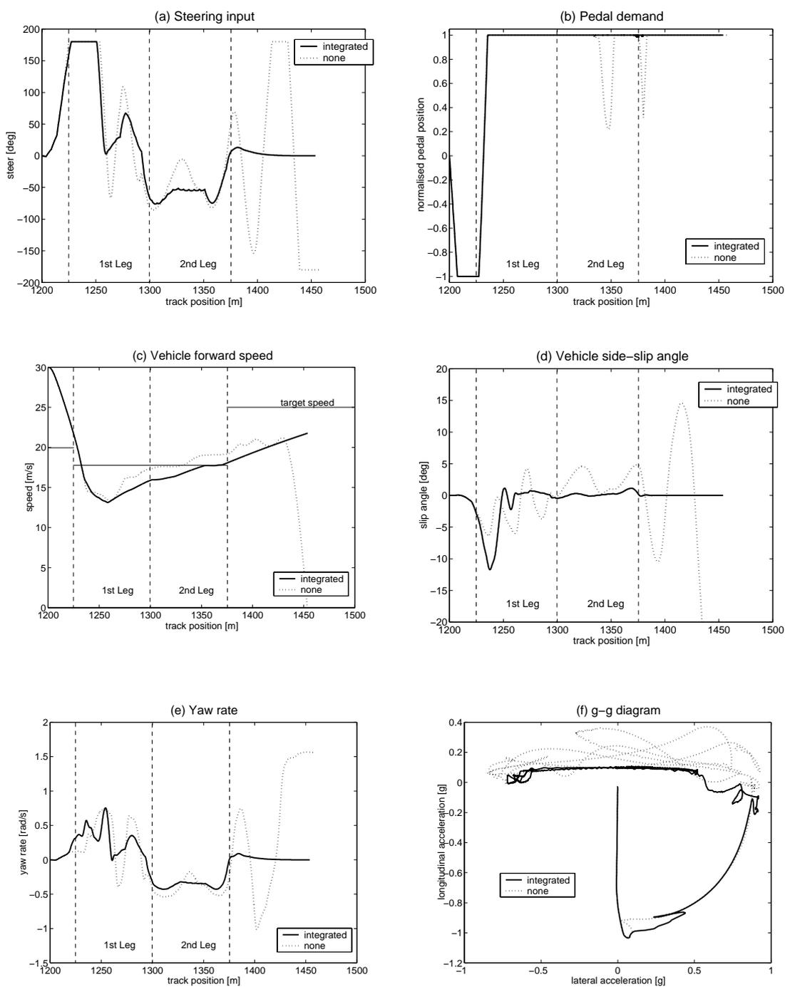
Fig. 15. Dynamic response effect of the integrated vehicle control system
