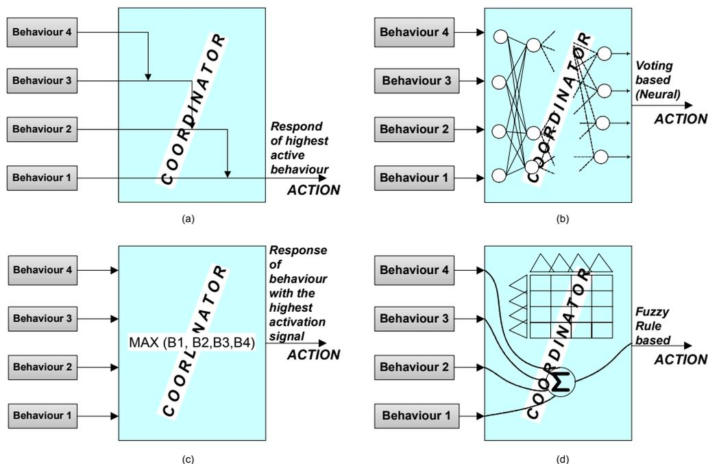
Fig. 12. Examples of control action coordination
