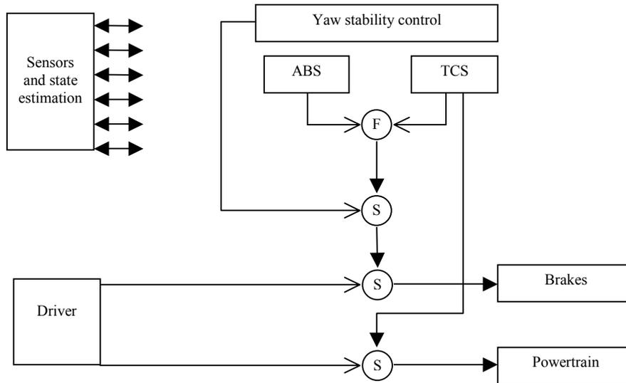
Fig. 13. Fuzzy coordinated control of vehicle dynamics
