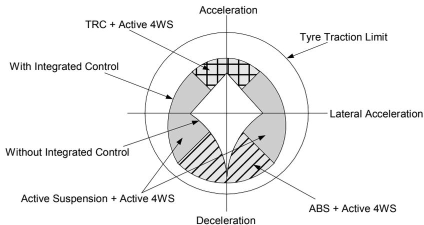
Fig. 2. Integrated Control and the g-g Diagram
