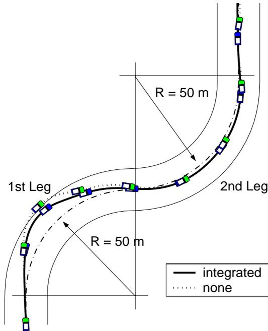
Fig. 14. Vehicle Path – severe braking through an S-bend
