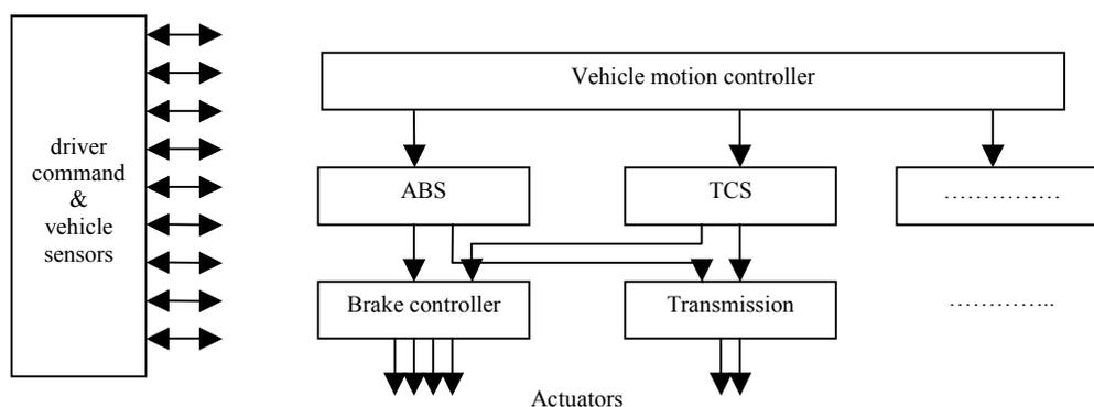
Fig. 9. Hierarchical Integrated Vehicle Control System
