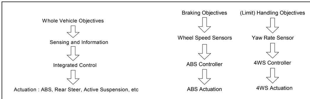
Fig. 4. Single versus parallel functional hierarchies
