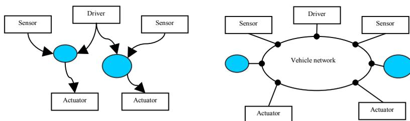
Fig. 3. Parallel versus network implementation of a parallel design topology
