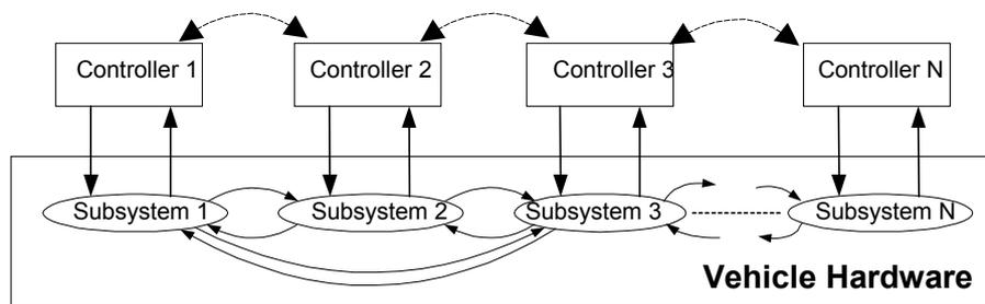
Fig. 7. Decentralised and heterarchical control
