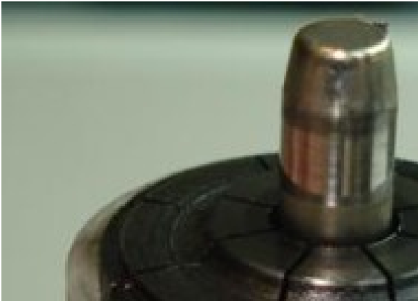
Figure 2. Example of Commutator Wear on a DC Motor
